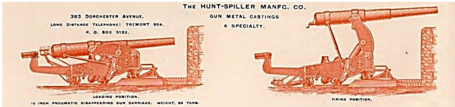
Hunt-Spiller letterhead showing a 66-ton pneumatically powered “disappearing” gun emplacement
