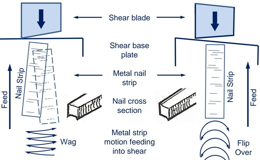
The shear is perpendicular to both the nail strip and its feed direction. By wagging the tail of the strip between cuts, the nail is tapered on its two sides. The head-end of the blank alternates between being on left and right sides, which is inconvenient for an automatic heading process.
